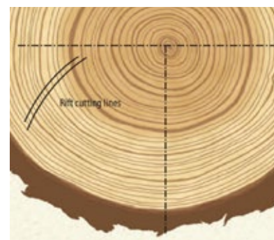
Logs are quartered and boards are sawn at an angle
