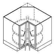
Doors can be adjusted independently of each other in all directions. Before making adjustments, make sure the corner cabinet is aligned exactly. If you use adjustable cabinet feet, special attention should be paid to adjusting the middle foot for support of the pole weight.
